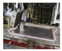
2-component polyurethanes for high pressure transfer moulding
