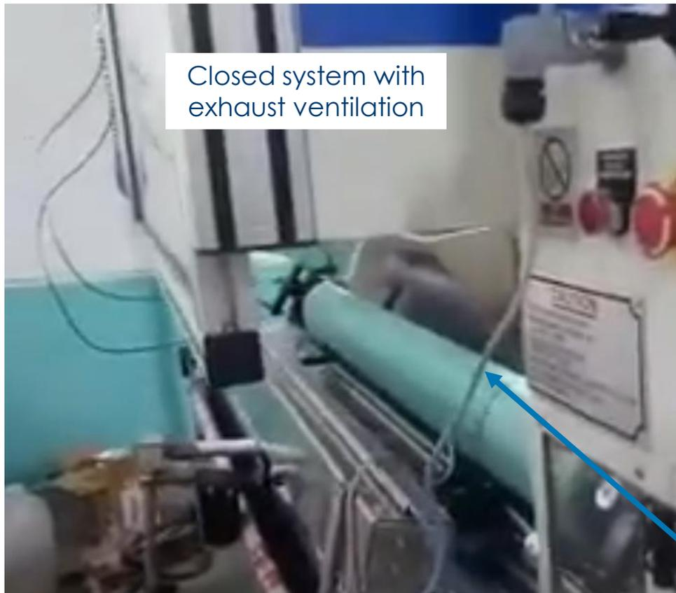
During operation, the operators are not exposed to the adhesive.
