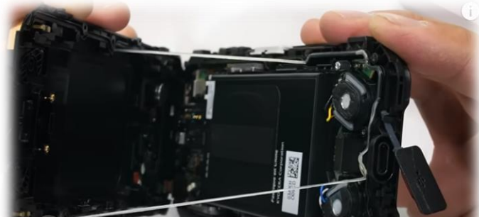
A sticky rubber gasket inlaid into a groove all around the edges → water-tightness
