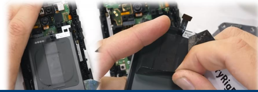
Removable 4500 milliamp hours battery with wireless charging permanently glued on the top
