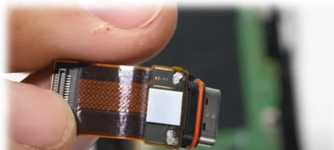
Charging port with its own red rubber ring → ingress protection
