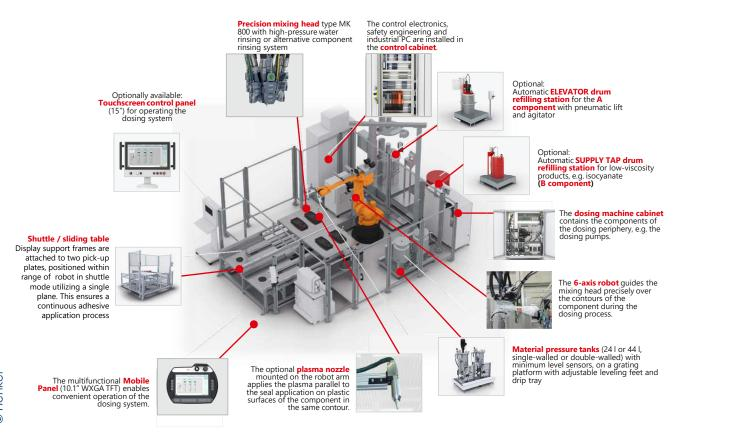
Depending on plastic used in support frame, plasma can be applied to contour of display frame beforehand to achieve an improved adhesive effect
