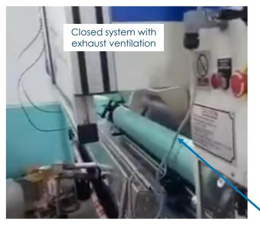
During operation, the operators are not exposed to the adhesive. Operators wear gloves and respiratory masks for a short period of time to manually clean the application station in typically < 15 minutes. Any adhesive waste dripping into a pan below the application station fully cures forming a cross-linked polymer not releasing any component of toxicological concern to human health and the environment.
