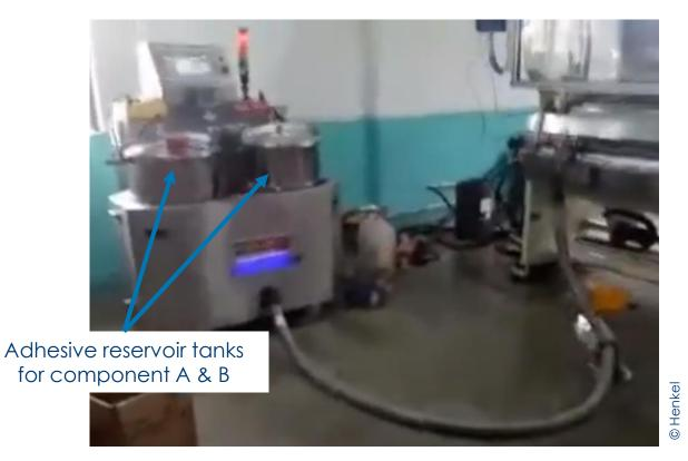
Operators wear gloves and respiratory masks for a short period of time to manually refill the reservoir tanks in typically < 15 minutes. During operation, the operators are not exposed to the adhesive.
