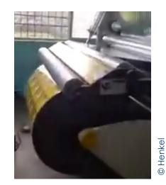
Laminate rewinding on a roll
