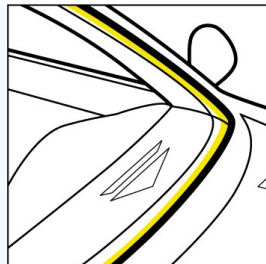
2. Direct glazing with and exterior bonding
