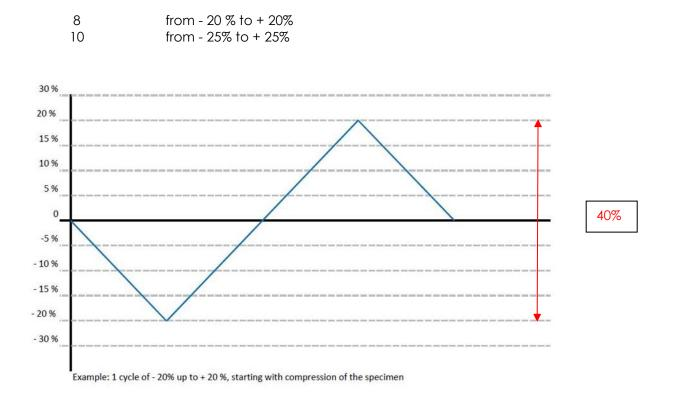
Additionally the specimen subjected to 1000 test cycles is evaluated visually:
