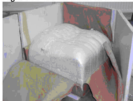
Figure 2: Cured foam in test box.
