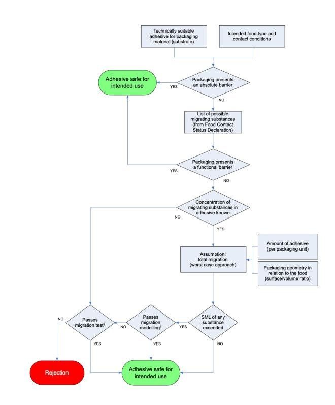
Figure 2. Flow chart for the assessment of the safe use of adhesives by the downstream user. (1. For example, using INRA ['Migresives' project], FABES MIGRATEST, SML Advanced of AKTS AG; 2. Internal or external testing, preferably at an accredited laboratory).
