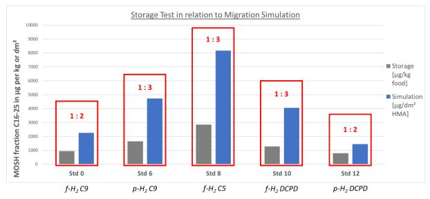
Figure 7: Results of storage test and migration simulation (MOSH fraction)
