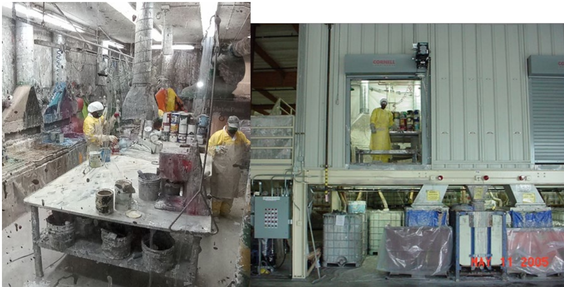
Figure 13: Photographs of some of the recycling steps ; Left: checking and opening the jars; Right: batching (source: MetroPaint)
