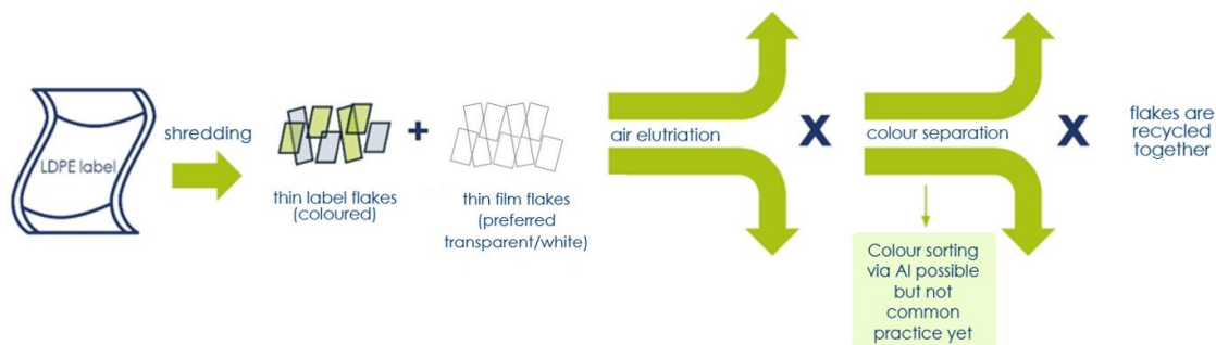
Figure 2: Inability to separate same-material released labels from flexible packaging.
