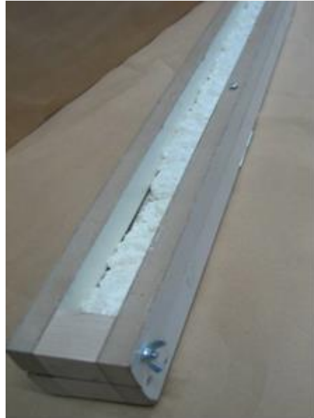
Figure 2: Setup with foam after application
