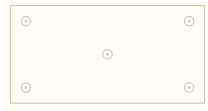
Figure 4: five anchors mechanical fixing system
