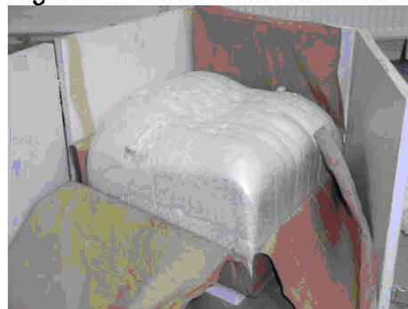
Figure 2: Cured foam in test box.
